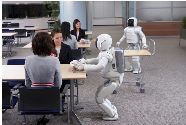
The robot Asimo has been developed by the Japanese Honda corporation. Here two robots are serving food. Asimo can recognise ten different people and address them by name. It can identify moving objects, people's posture and their gestures. Photo: Honda
